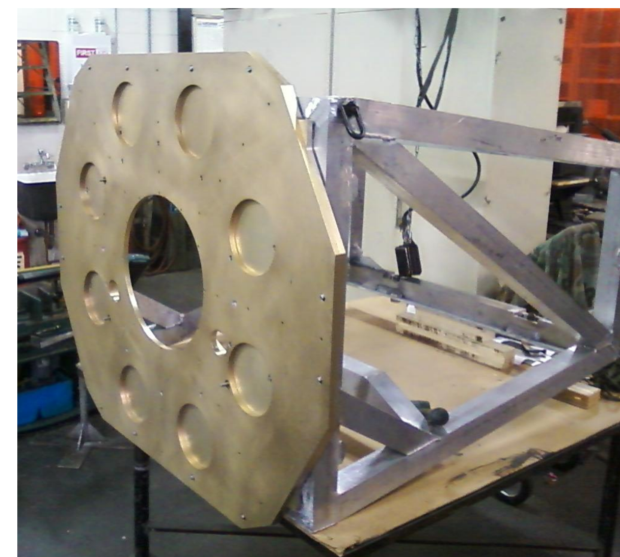
The adapter plate is mounted to the Nasmyth port of the telescope first, and then the main instrument structure is mounted to this plate. Alignment pins ensure repeatable installation.
