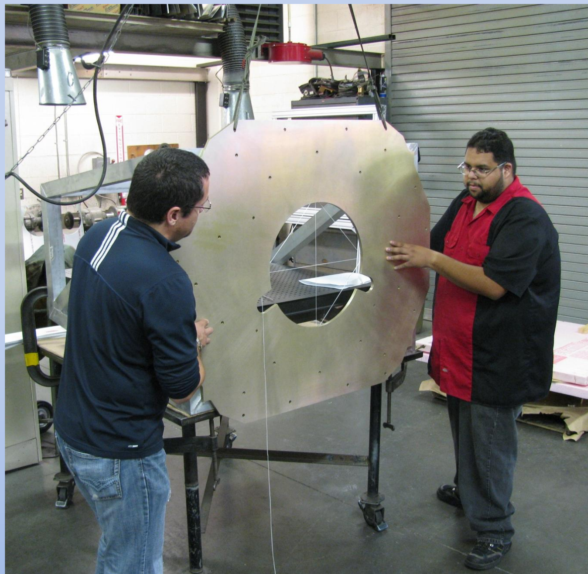
Adjusting the plate in height, left-right position and clocking relative to the frame and optical table.
