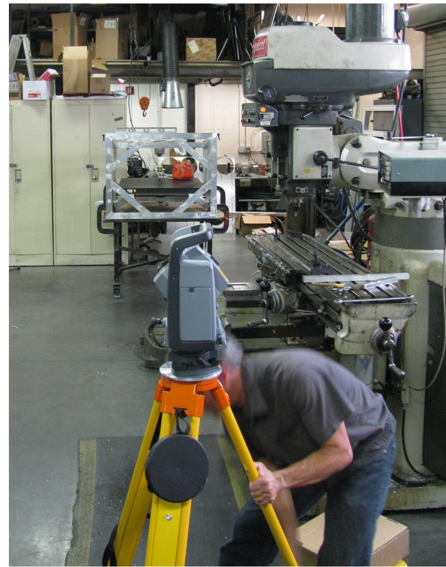
Setting up the total station that is used to sight along the mounting holes of the optical table and then align the mounting plate to the frame.
