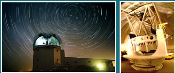
Figure 1. The Magdalena Ridge Observatory 2.4-meter fast-tracking telescope (right) and support facility (left) located outside of Socorro, NM on Magdalena Ridge at 10,612 feet. The observatory became operational in September 2008, and performs target-of-opportunity scientific research as well as work in the area of space situational awareness.
